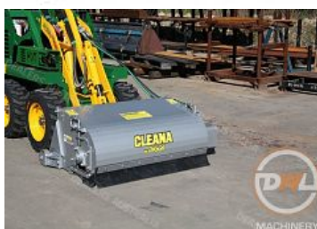
Hi performance forward and reverse bucket broom.
