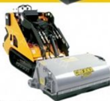
Hi performance forward and reverse bucket broom.
